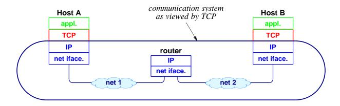
• TCP on one computer uses IP to communicate with TCP on another computer
